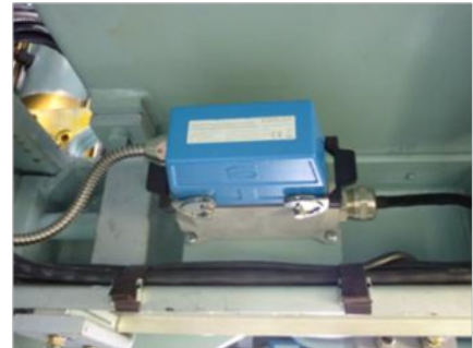
Kistler sensor on engine in operation
